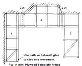
Note: A cross-member should be placed where a seam is to be made.
