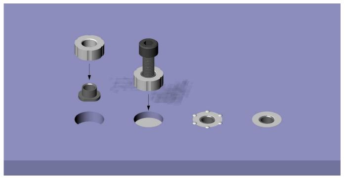
Squirrel® Fixings have been developed to allow fabricators to make a mechanical screw fixing into a 12mm sheet of Corian®. The insert is recessed a maximum of 8mm into the back of the sheet to prevent it from being visible through the face side. Please note that the inserts will be visible through translucent colours.
