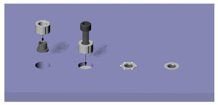
Squirrel® Fixings have been developed to allow fabricators to make a mechanical screw fixing into a 12mm sheet of Corian®. The insert is recessed a maximum of 8mm into the back of the sheet to prevent it from being visible through the face side. Please note that the inserts will be visible through translucent colours.
